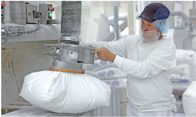
JumboSprint EX for handling bags in an explosion protection zone
