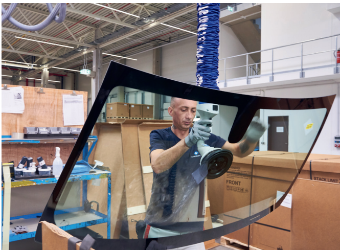
Vacuum tube lifter JumboFlex for handling windshields
