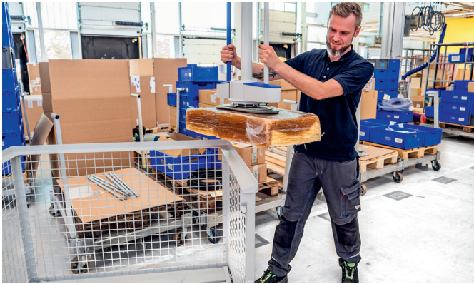
Jumbo Low-Stack for handling raw rubber bales in grid boxes
