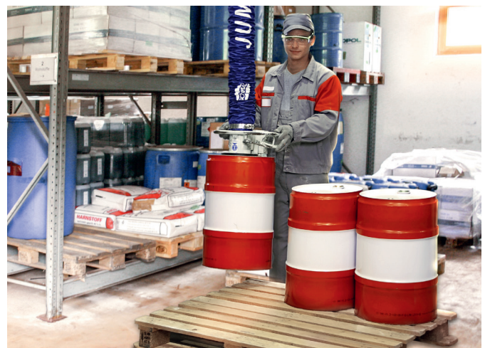
Vacuum tube lifter JumboSprint for handling barrels
