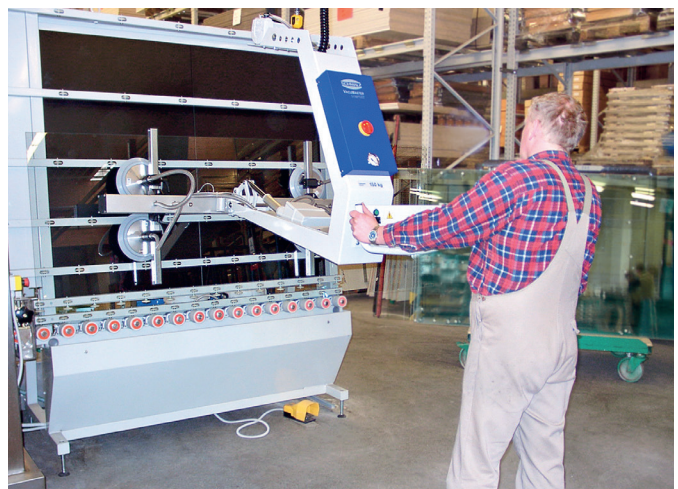
Vacuum lifting device VacuMaster Comfort for turning a glass sheet by 180°
