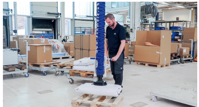
JumboFlex High-Stack when handling bags
