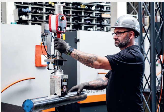
Quick-Lift Rail for intuitive and ergonomic load movement
