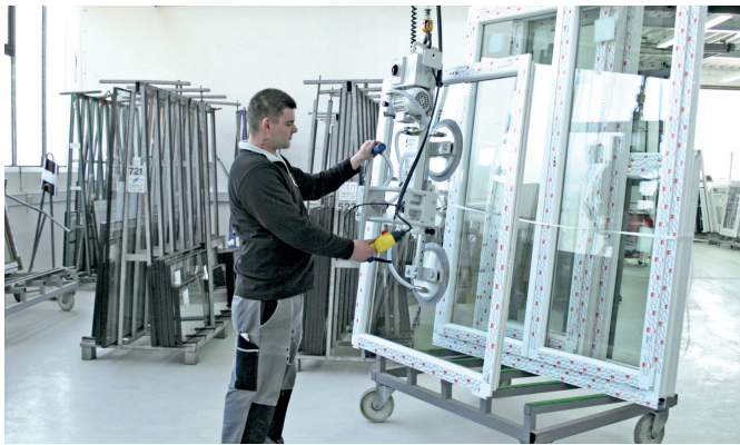
VacuMaster Window for rotating and palletizing windows
