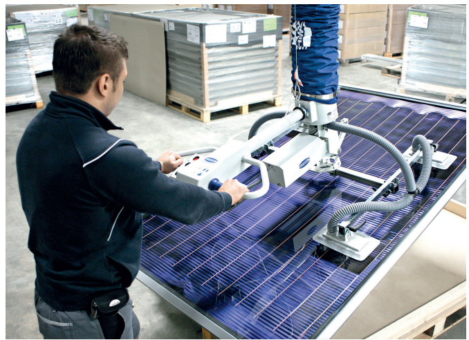
Solar | Vacuum tube lifter JumboErgo with 90° swivel angle for handling solar panels
