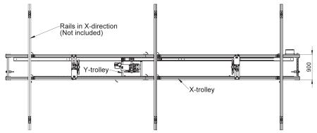
The rail system, Quick-Lift Driven 300i (QLD 300i) is a unique, motorized lifting device that easily covers large areas horizontally, with a lifting load up to 300 kg.
